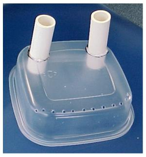
A plastic cover was added to the aquarium to prevent water evaporation as well as any splattering of the heavy metal.
