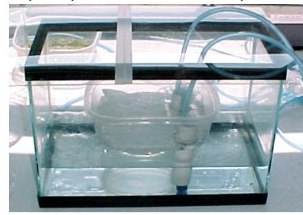
The amount of copper remaining after the test period was 4.6 p.p.m. Subtracting this from the initial concentration of 20 p.p.m. we find that 15.4 p.p.m. of copper has been absorbed by the mustard seeds. Multiplying 15.4 times the 3 liters of water in the aquarium gives us 46.2 milligrams of copper that has been removed. Dividing by
